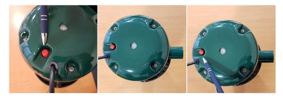
Following a Jam, check the rotor can be turned manually in both directions with the de-jam key, then press the red reset button at the base of the unit, you need to give the reset a firm upwards push and if the unit needed resetting you will hear a "click" making sure the reverse switch is to the left or the right as the centre is off and then try activating the unit again.
