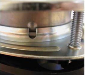
Next, (Slot.gif) you should be able to see that the 3 bolts holding the hopper to the sink bush assembly are all the way into the slots. You may have to take a nut and washer off to see clearly
